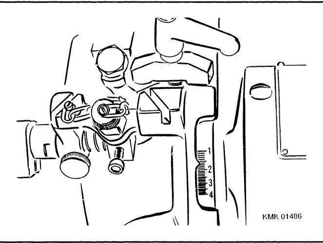
Shut off high pressure and switch off test bench.
